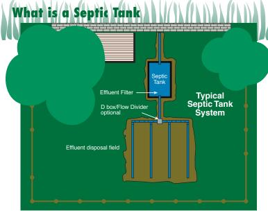
Septic tank systems are individual wastewater treatment systems that collect, treat and dispose of wastewater. They are reliable, cost effective and efficient. Septic tank systems are used where municipal sewers are not available or are impractical.
